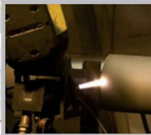
A thermally sprayed surface treatment is applied to replace hard chrome plate for improved wear and corrosion resistance.
