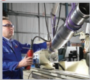
The component is surface machined using diamond tools due to the extreme hardness of the surface finish.
