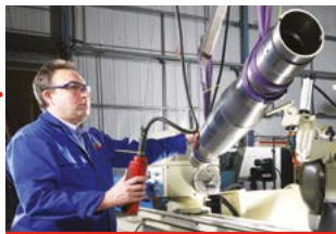
B The component is surface machined using diamond tools due to the extreme hardness of the surface finish.
