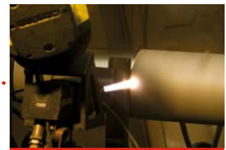
B A thermally sprayed surface treatment is applied to replace hard chrome plate for improved wear and corrosion resistance.
