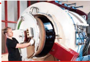
B The part is heat treated to harden and temper the steel.
