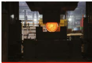
Alloy steel billet is forged to shape.
