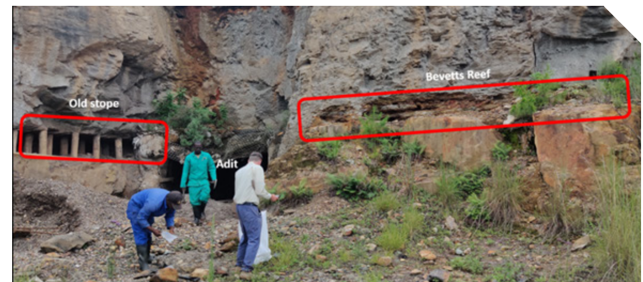
Figure 10: Sampling at the old Frankfort Mine, Bevetts Reef, Beverly Hills area. Grades up to 3.2 g/t Au recorded.
