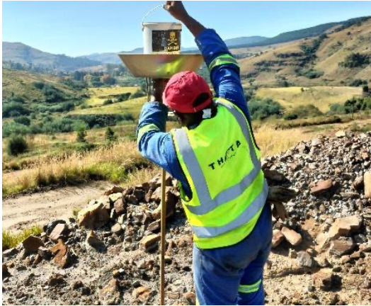
Figures 15: Dust fall sampling at Tailings Storage Facility at TGME Gold mine
