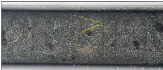
Photo 2: RKDD002-626.5m: Pyrrhotite, trace pentlandite/chalcopyrite in cumulate textured ultramafic
