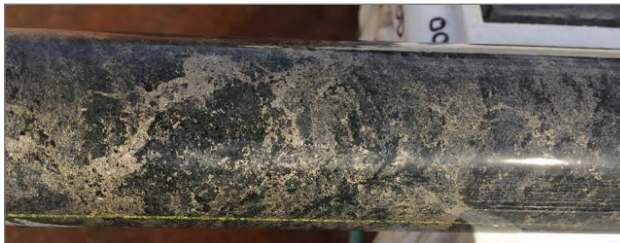
Photo 1: RKDD001-566.8m: Pyrrhotite in metasediment (granulite)
