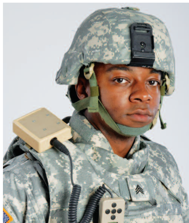
The acoustic EARS® family of wearable, sniper detection and gunshot localisation solutions is based on a miniature single integrated acoustic sensor
