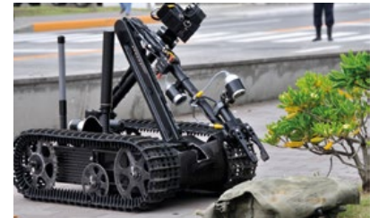
A Mk. II TALON robot from Japan-based Explosive Ordnance Disposal Mobile Unit 5, is used to inspect a suspicious package during a force protection and anti-terrorism training exercise at a United States Navy base in Japan. The exercise trained first responders and support personnel how to react to an improvised explosive device scenario.
