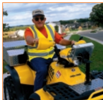
Leak detection equipment on an all-terrain vehicle allows Harold Johnson, MGE Lead Leak Survey Serviceman, to inspect gas lines in areas unreachable by truck. The American Gas Association recognized MGE as a leading performer in monitoring and maintaining its gas system.
