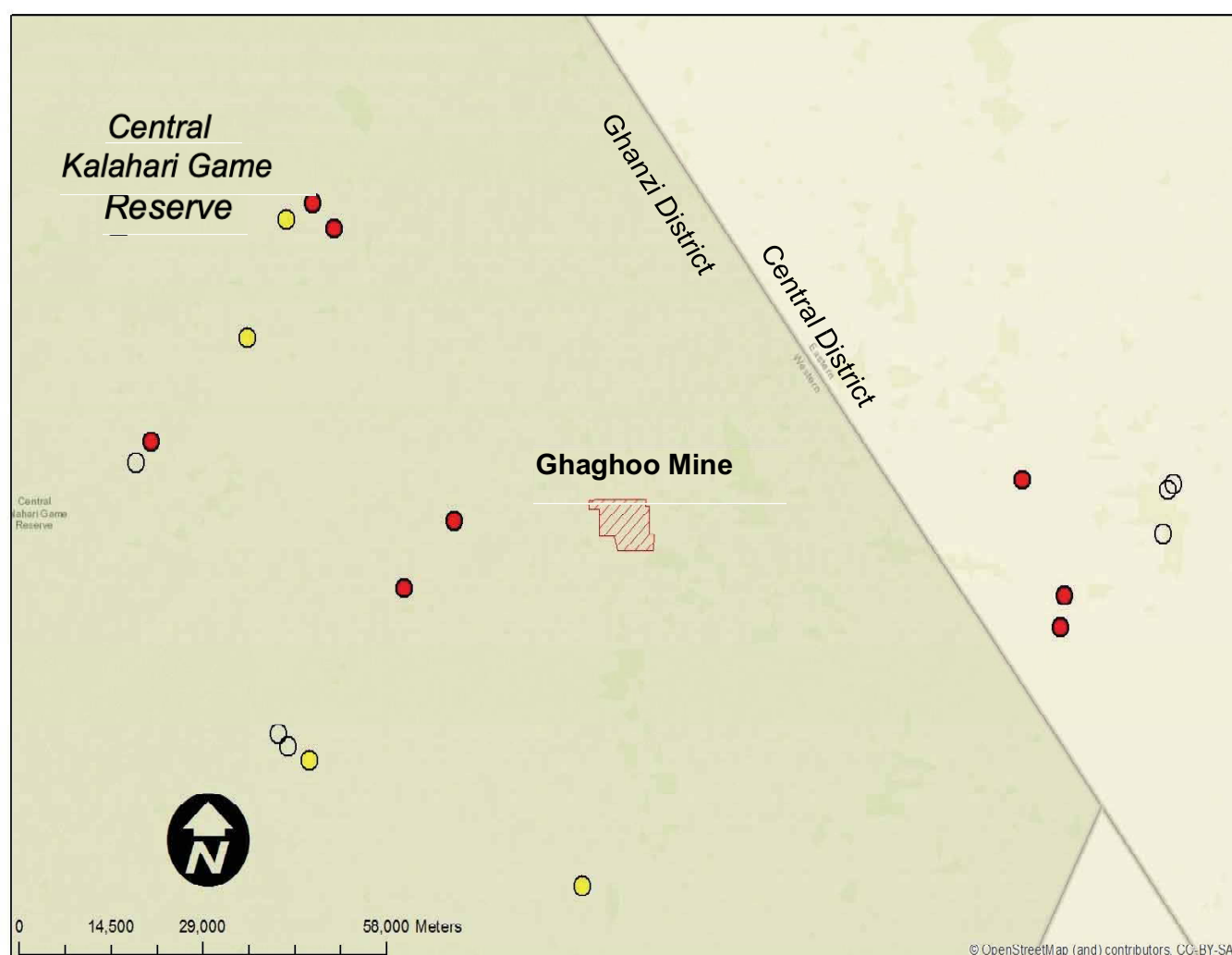
Figure 7: Location of high priority aeromagnetic targets (Red = 8 high interest targets; Yellow: low priority targets; Black empty circles: targets discarded on the basis of poor walk magnetic response)
