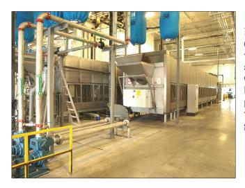
Highly automated and energy efficient dryers (above) combined with twin 16 chamber tunnel washers (left) enhance production efficiencies and processing quality to a very high level. Combined with a labour saving materials handling system via overhead monorail, the new plant has the capacity to handle additional volume available now and in the future in a growing southern Alberta market.
