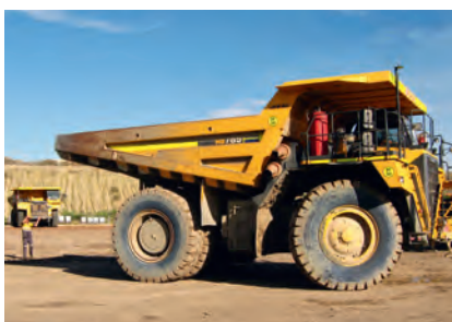
Larger mining haul trucks increase fuel efficiency at Ellendale
