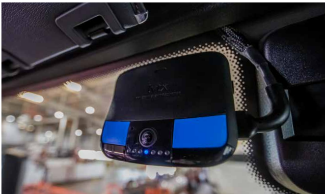
An inward-facing camera installed in one of our trucks
