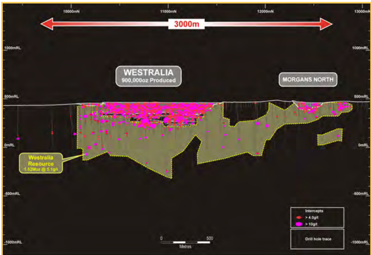
Figure 9: Long section of the 1.5 million ounce Westralia Mineral Resource, mine workings and drill holes. The image represents a south (left) to north (right) long section. The resource exhibits continuous mineralisation over a distance of 2.8km, and remains open at depth.
