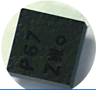
Electronic compass The electronic compass was devel- oped by combining Hall elements, LSIs to amplify the sensor signals, and signal-processing software algorithms.
