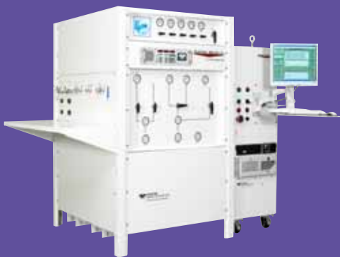
Teledyne Energy Systems new Medusa LS fuel cell test station can test fuel cell stacks at power levels up to 10 kilowatts, a common test range for developers of automotive power systems
