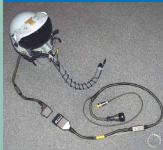
Teledyne Reynolds developed proprietary high-voltage connectors and subassemblies for the Joint Helmet Mounted Cueing System, which gives pilots the ability to designate a target simply by looking at it
