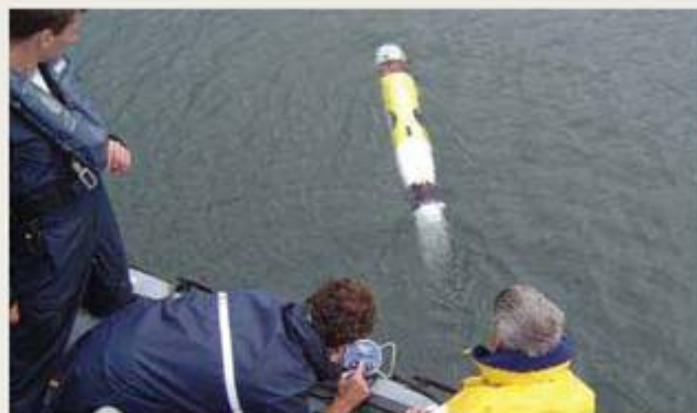
A Teledyne RD Instruments Long Ranger Acoustic Doppler Current Profiler is deployed from an offshore platform. The Long Ranger is used extensively to monitor potentially dangerous deep water currents surrounding offshore oil and gas platforms.
