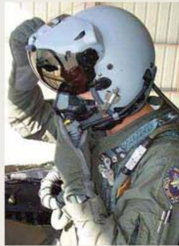
The Teledyne Reynolds' Joint Helmet Mounted Cueing System cable assembly extends from the rear of a pilot's helmet, over the left shoulder, and interfaces with the aircraft avionics system.
