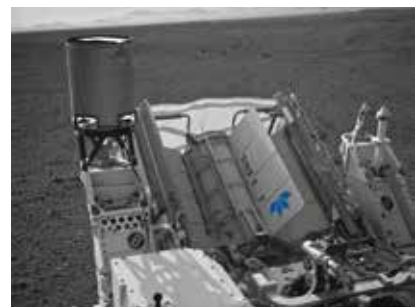
Taken with Teledyne DALSA-built image sensors, this photo shows Curiosity's radioisotope thermoelectric generator, built by Teledyne Energy Systems.
