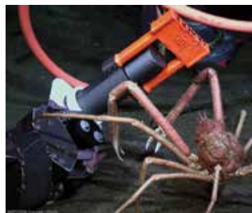
Teledyne's wet-mate electrical and fiber-optic interconnect systems allow installation, maintenance, and upgrade of subsea networks in the harshest environments. Photo credit: UVic NEPTUNE
