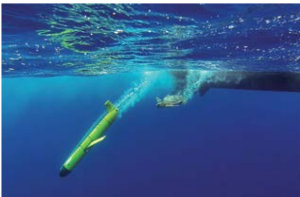
Pictured above is Teledyne's Slocum® Glider, which measures oceanographic data that help scientists study the health of the ocean.
