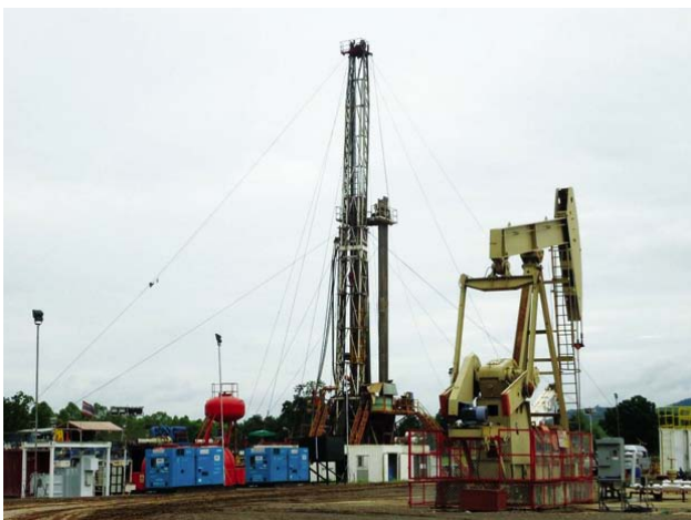
Figure 6. Small footprint, easily transportable drilling rig.
