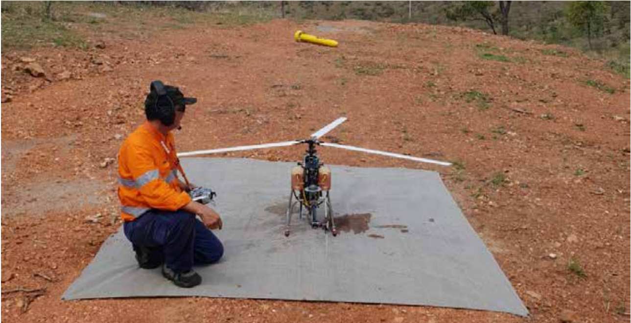
Drone technology for Magnetic survey deployed at the Drummond project
