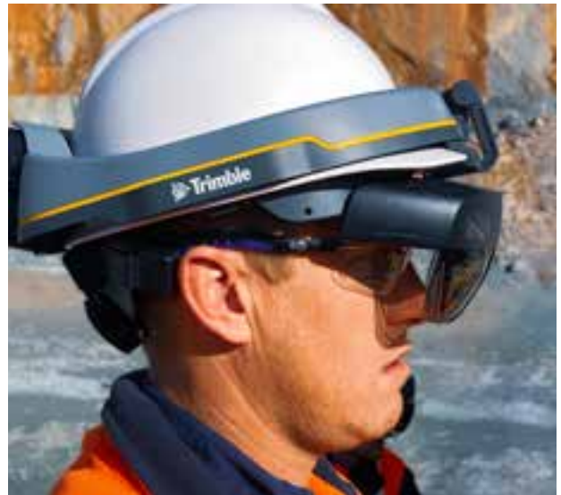
Hololens (Augmented Reality) technology at Cowal - enables maintenance teams on the surface and/or at the Original Equipment Manufacturer or Dealership to view what the maintainer is seeing in real-time to expedite troubleshooting eg working on an excavator in the open pit
