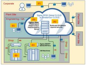
Figure 1. Sigma's Industrial IoT / PrintRite3D® Cloud Architecture
