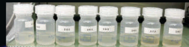
FIGURE 2: ELECTROLYTE SAMPLES SHOWING DISCOLOURATION – LEFT TO RIGHT, 4N ALUMINA (99.99%), 3N ALUMINA (99.9%), BOEHMITE (99.7%)
