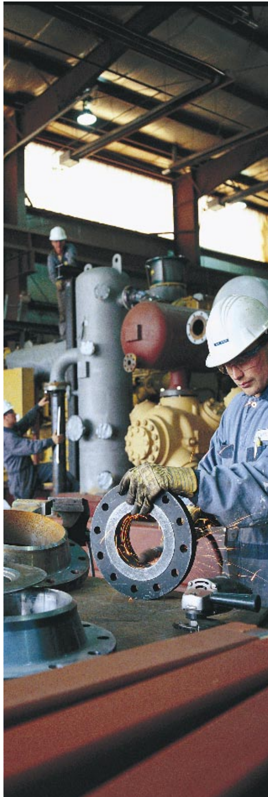
Energy Industries employees assembling natural gas compression units
