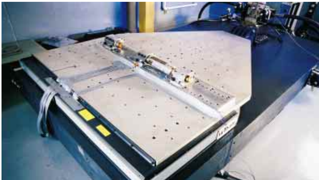
On Advantage's vibration table, tools or components of tools are tested to evaluate their durability.
