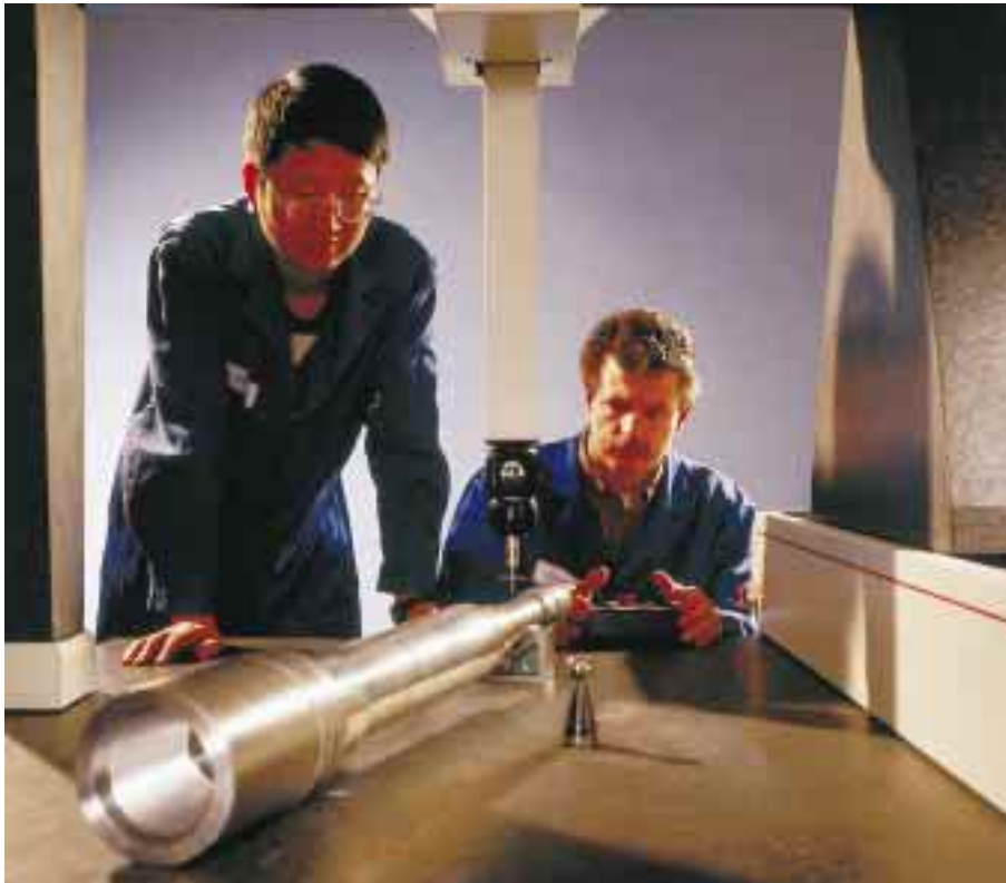
A specialized laser measurement instrument ensures exact tolerances in the manufacture of completion tools.
