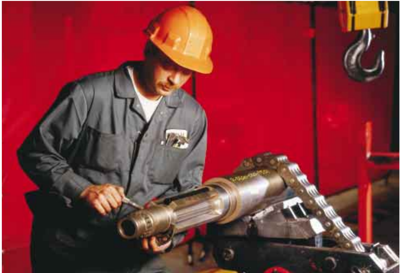
After each rental, the torsional shock tool is inspected and redressed.
