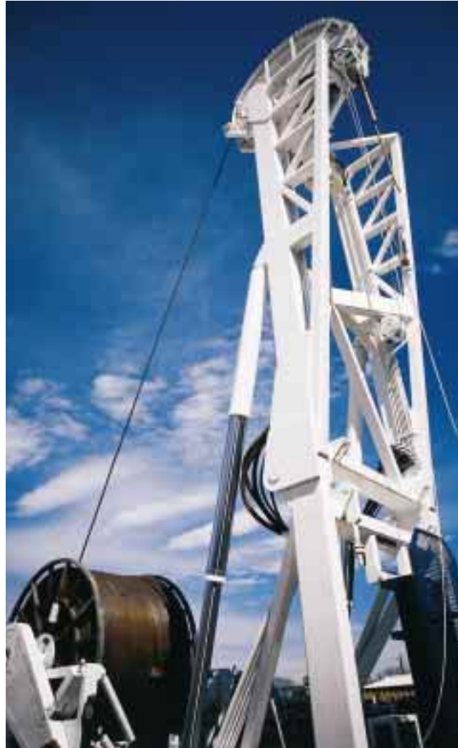
Continuous coiled tubing, our newest drilling technology.
