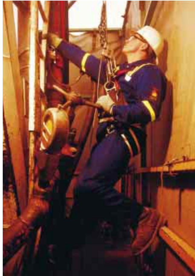
Fall arresters save lives. A derrickman attaches his safety harness to the fall arrester prior to his ascent up the rig mast to the monkey board.
