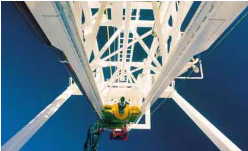
On our Super Single™ rigs, the top drive travels along a track system built into a one piece mast which can be set to varying degrees, from vertical to a 45 degree slant position.
