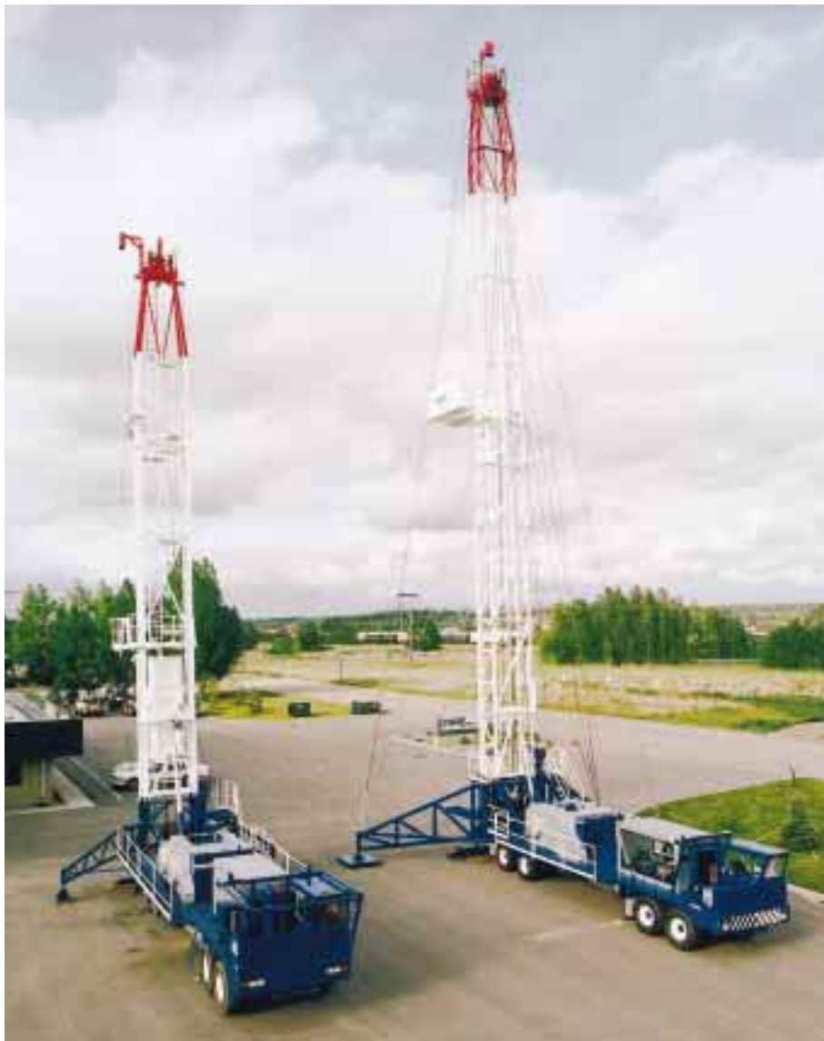
The batwing design, as illustrated on rigs 607 and 609, eliminates the need for guy wires to anchor the rigs' masts prior to the start of operations.
