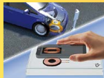
Wireless power transfer technology for EVs (top) Wireless power transfer for ICT equipment
