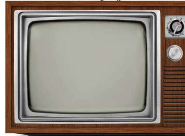
Common black-and-white consumer TV set As consumer TV sets became extremely popular during the high economic growth period, ferrite from TDK was extensively used as a core material for deflection yokes on cathode-ray tubes. The move toward bigger screens was also supported by improved performance of the deflection yoke cores.
