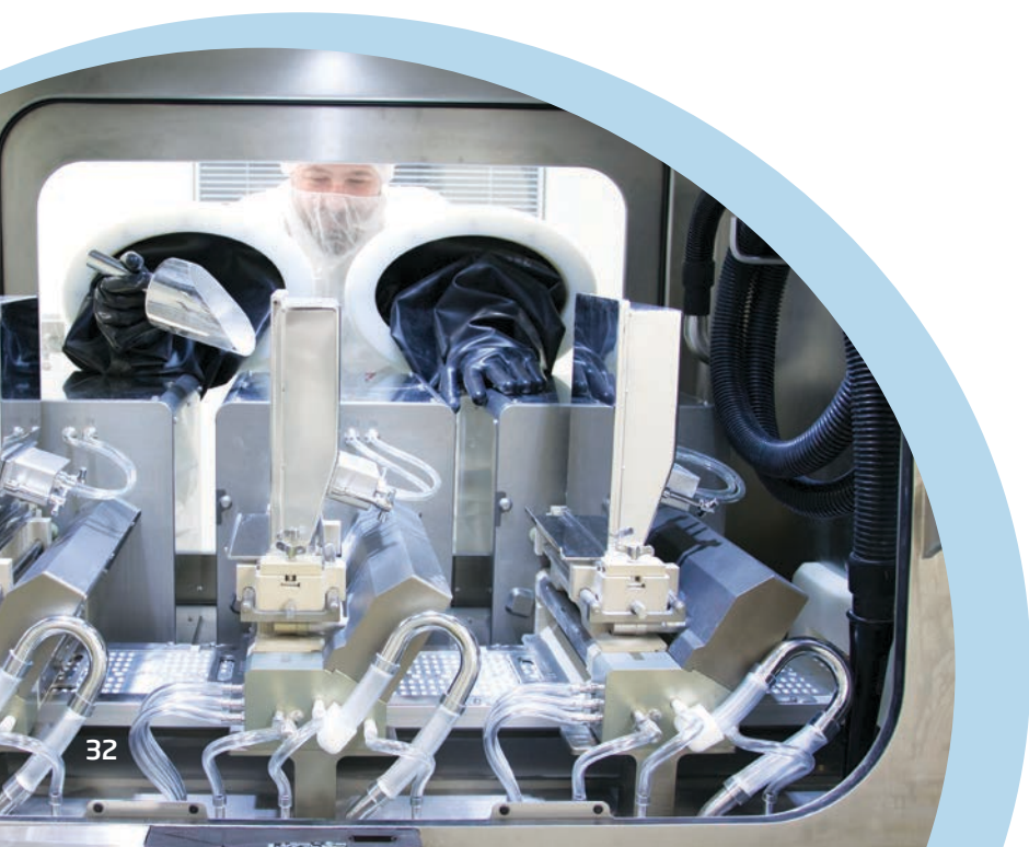
Powder dosing modules on high speed blister filling line
