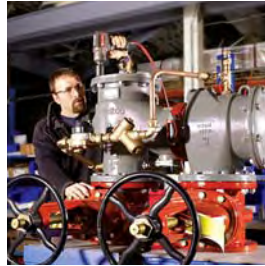
Final Assembly of a FEBCO Backflow Preventer
