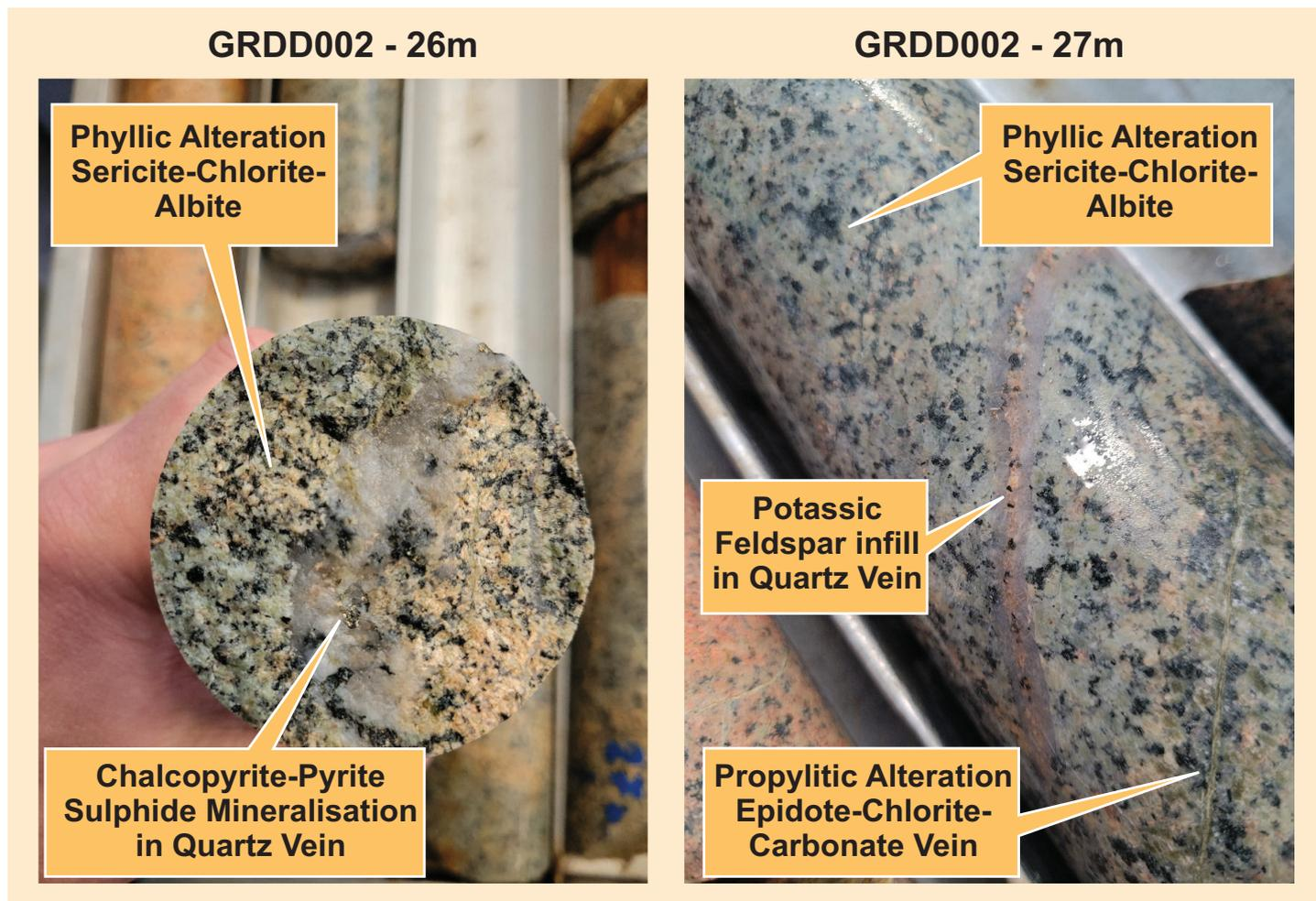
Figure 8: Photos of drill core from GRDD002 showing A: quartz vein mineralisation, visual estimate of 0.2% copper mineralisation and B: multiphase alteration styles in unsampled core at the NSW Core Library.
