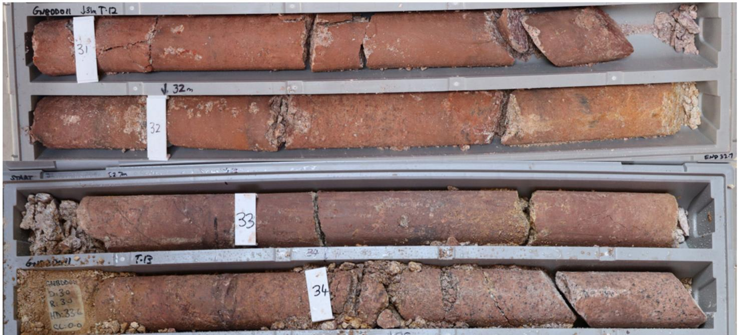
Figure 2: Photo of a section of drill core from GNBDD011, showing the clays and is host to 3m at 3,481ppm TREO from 31m, this interval sits within the larger interval of 27.4m at 1,426ppm TREO from 26m downhole
