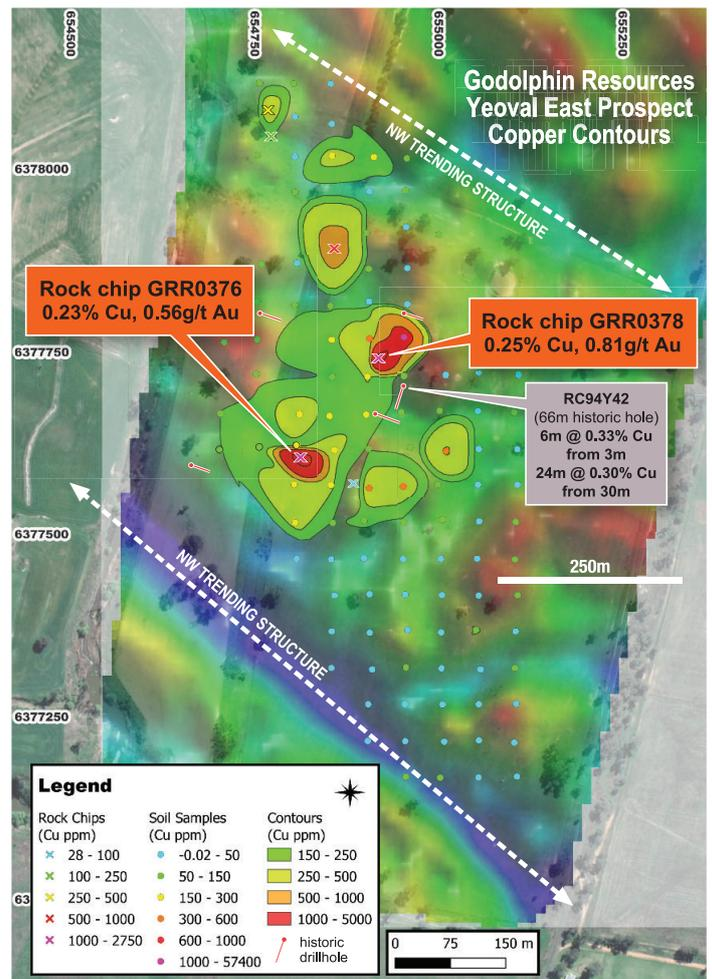
Figure 9. Contoured >150ppm copper soils & rock results over TMI ground magnetics imagery, Yeoval East Prospect.
