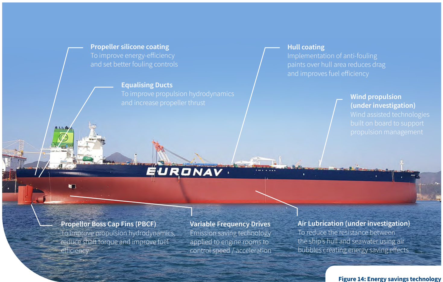
Figure 14: Energy savings technology
