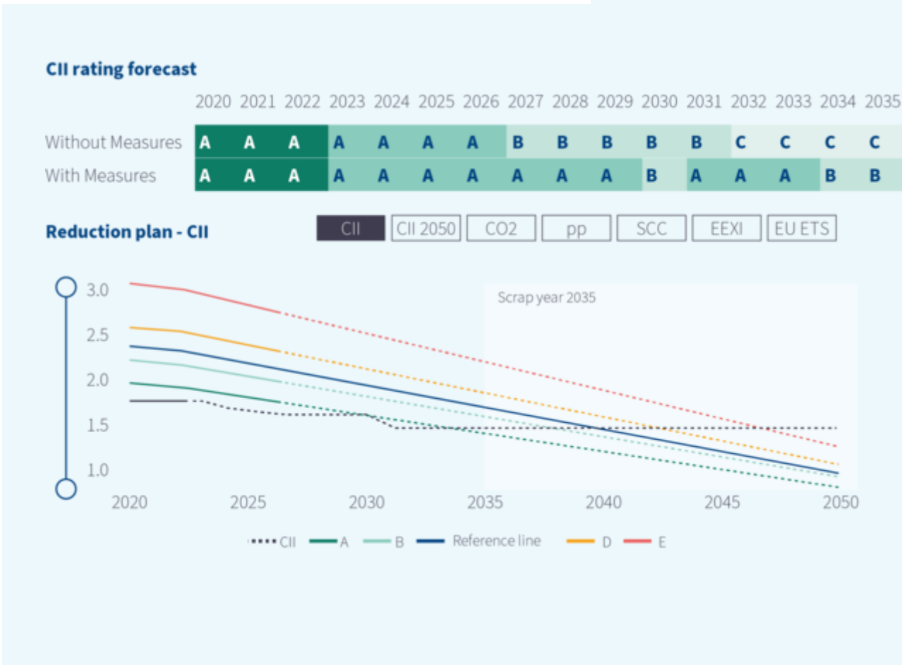
Figure 17: CII rating forecast for vessel Dia (VLCC - 2015) - with and without measures.
