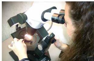
In GCAL, technology is employed in every phase to verify natural and synthetic, identify inclusions for clarity, examine color variances, produce Sarin measurements, provide Spectrometer measurements along with other techniques.
