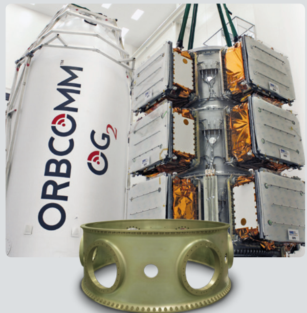
Satellite constellation installed onto the Moog ESPA Courtesy of ORBCOMM
