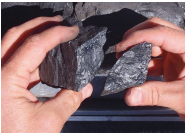
Figure 6. High quality thermal coal in large diameter core from the Mmamabula West A-Seam
