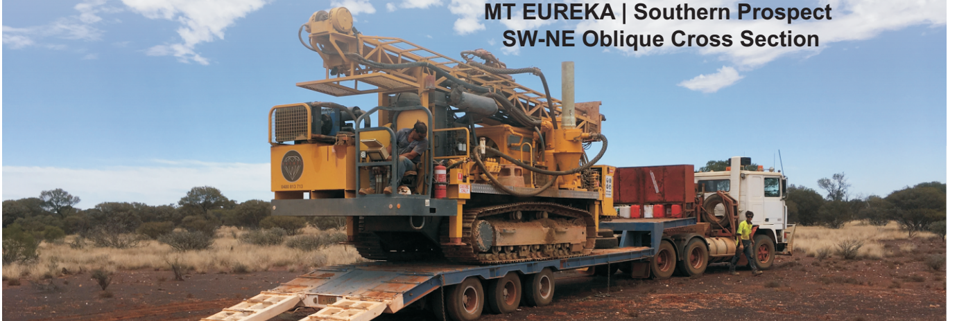
MT EUREKA | TRACK-MOUNTED AIRCORE DRILL RIG
