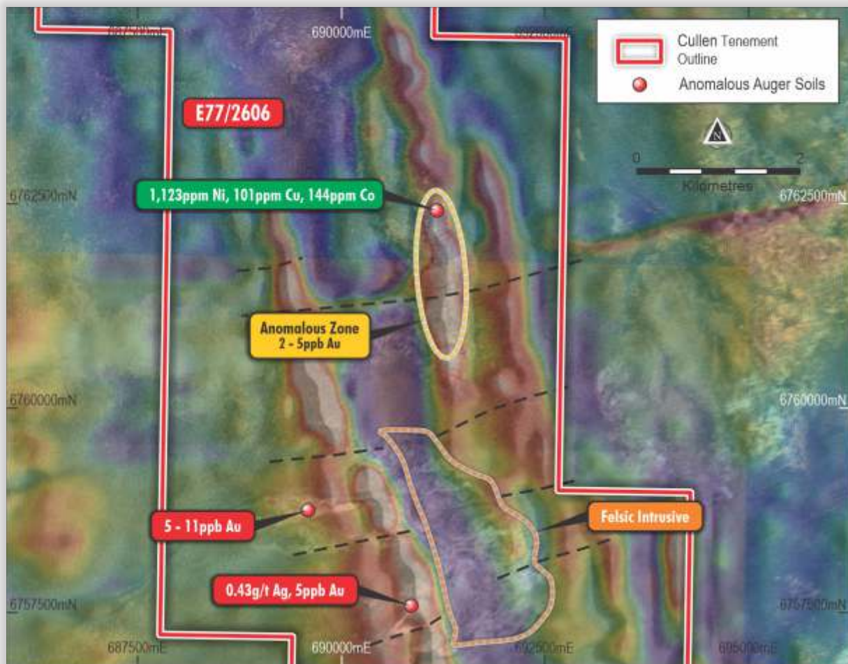
BARLEE PROJECT | Geochemical anomalies from auger sampling (ASX: CUL;8-3-2021) along interpreted, gold-prospective Youanmi Shear Zone corridor (yellow arrows), cut by east-west breaks
