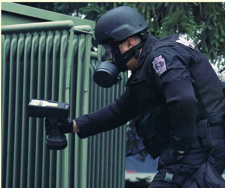
The HAZMATCAD™ Detector provides law enforcement officials with a new tool for fighting the war on terror. Utilizing surface acoustic wave technology, it can quickly detect and classify trace amounts of chemical warfare agents.
