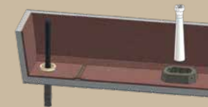
'Ladle to Mould' configuration
