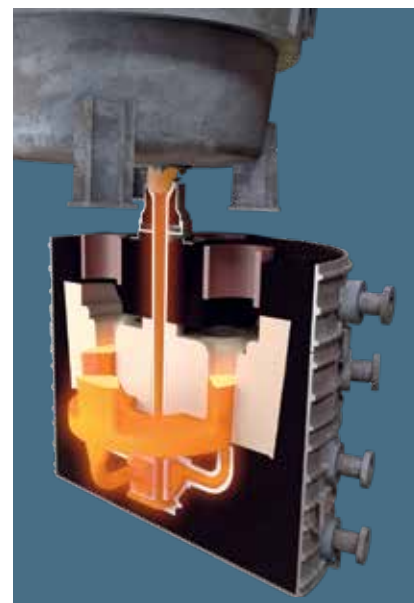
Pouring a steel casting using the Hollotex Shroud
