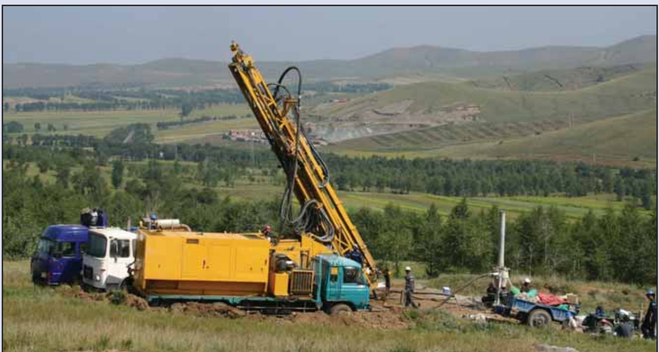
RC DRILL RIG ON ZONE II SUMMER 2005
