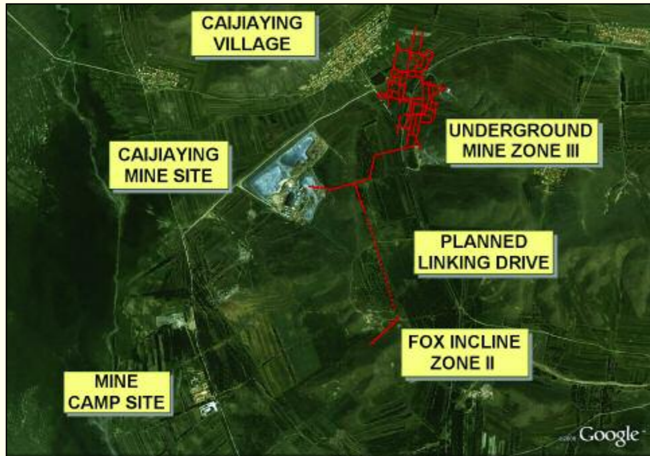
Superimposed Diagrammatic View of Underground Mine Workings at Caijiaying: Courtesy of Google Maps
