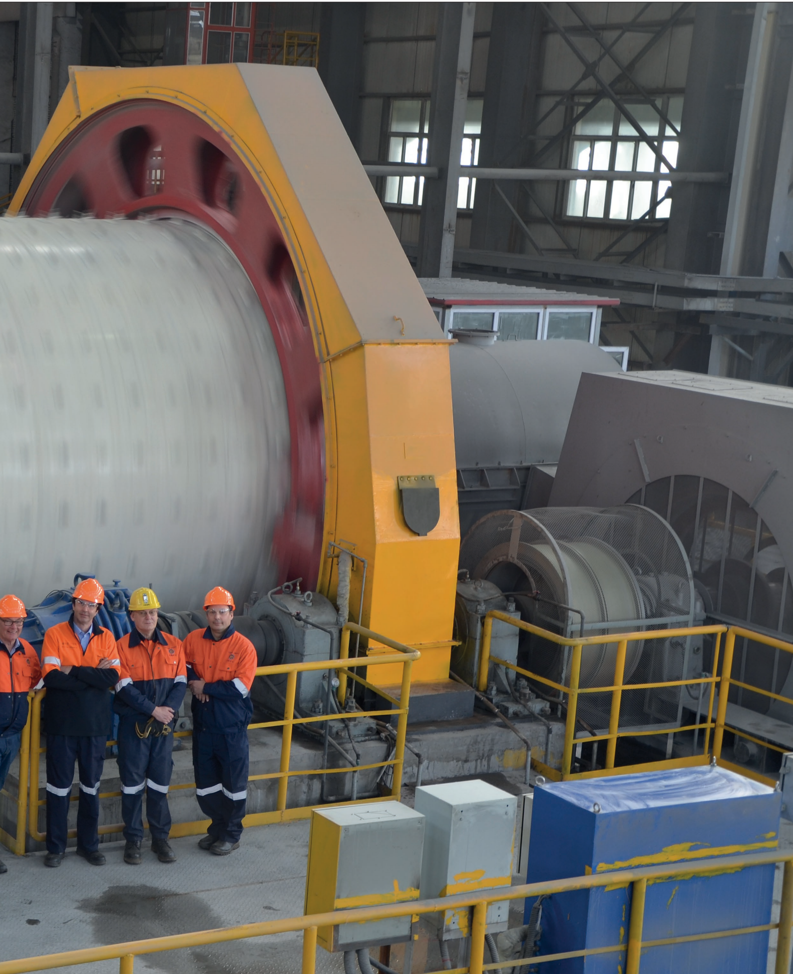
Griffin Directors Rupert Crowe, Dal Brynelsen Mladen Ninkov, Roger Goodwin and Adam Usdan by the newly commissioned 750,000 tonne per annum primary ball mill
