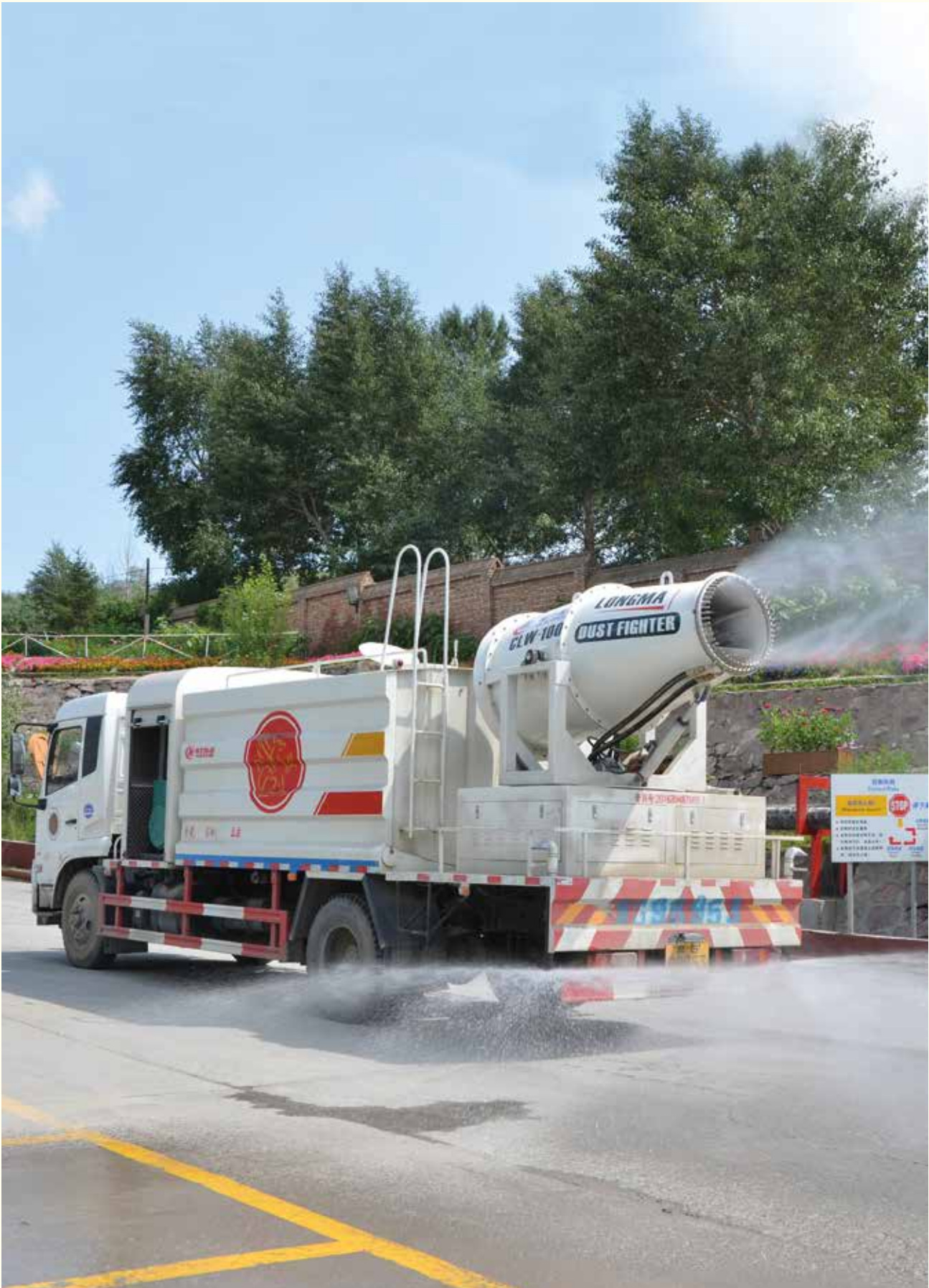
Dust Suppressor in Operation at the Caijiaying Mine
