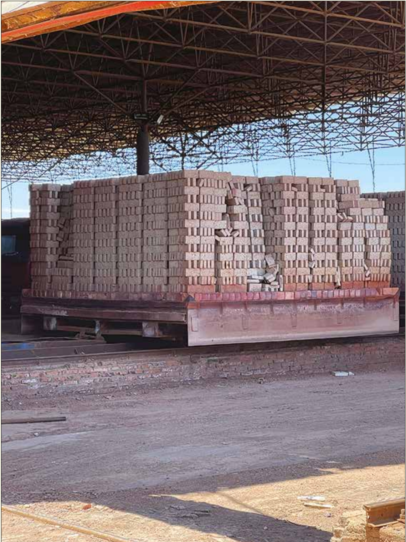
Bricks manufactured from recycled tailings from the Caijiaying Mine
