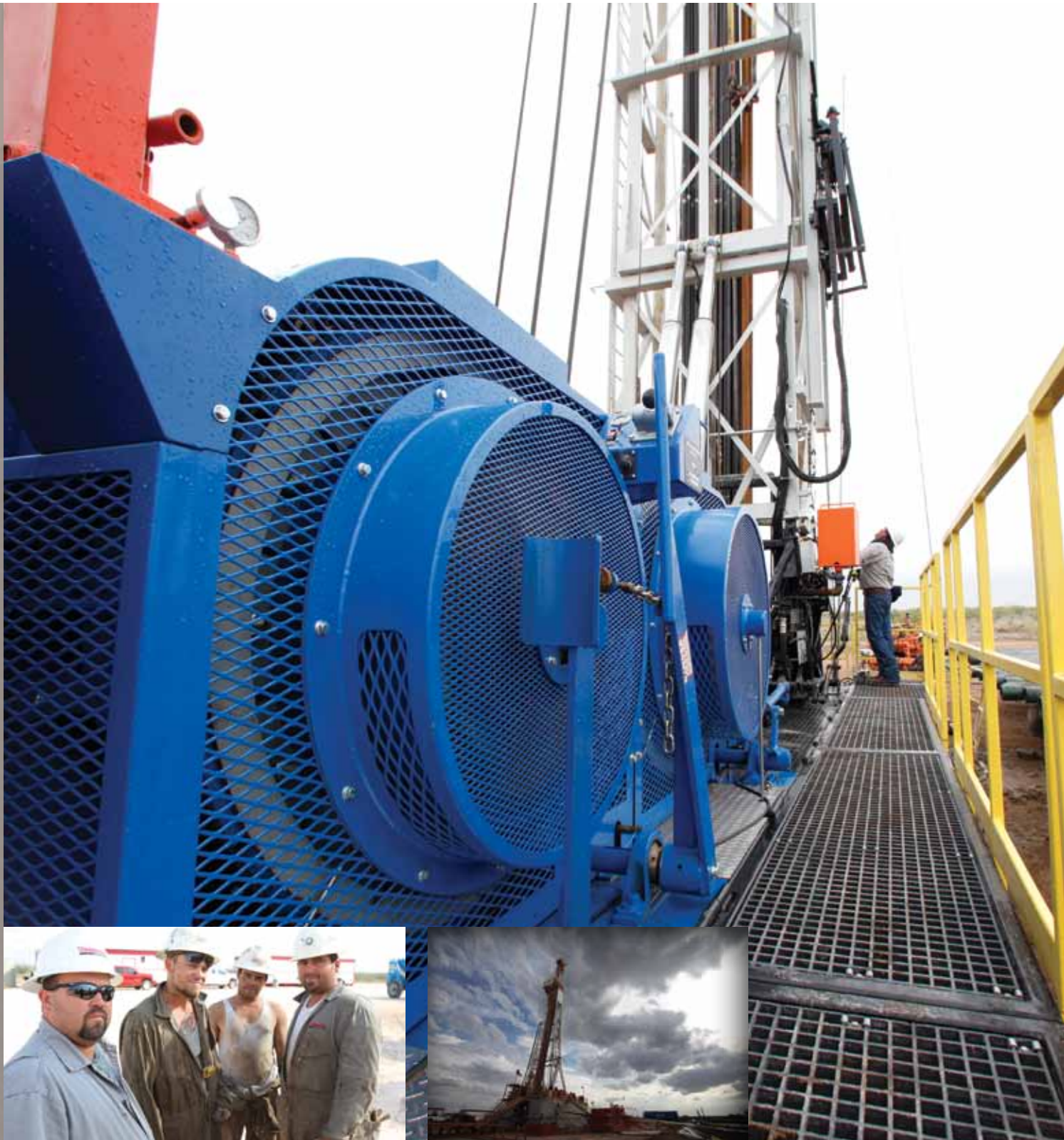
LOCATION: Odessa/Midland Oil Fields, Texas, USA — — EQUIPMENT: Twin Disc PO-124, PO-324, and PO-108 Air Clutches
