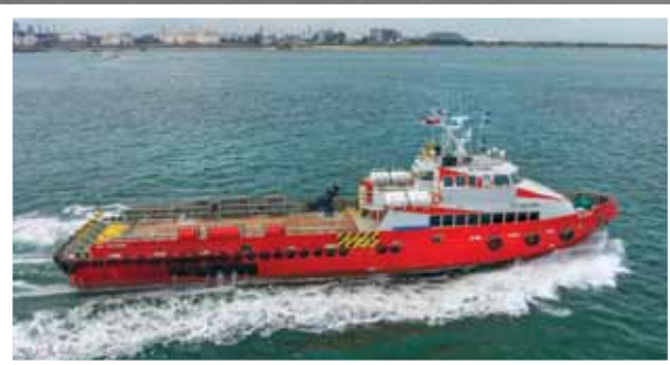
LEFT - Built for speed and security by Penguin International Limited, Singapore, the FLEX-40SL multi-role, 131-foot (40-meter), aluminum-hulled MV Ashley achieves 27 knots with its three 1350-hp (1007-kW) Cummins engines driving through MGX-6690SC QuickShift® transmissions complemented by an impressive array of Twin Disc products including EC300 controls, Twin Disc shafts, rudders and Rolla™ submerged propellers.
