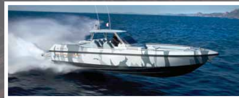
LEFT - The glass Kevlar®/carbon-hulled Couach Hornet 1300 (42 feet/13 meters) can attain 52 knots with its twin MAN 800-hp (597-kW) engines working through Twin Disc QuickShift® marine transmissions to drive Arneson ASD11 Surface Drives™ with Twin Disc trim tabs and Rolla™ Propellers.
