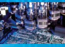
Surface mounting lends itself well to a high degree of automation, reducing labor costs and greatly increasing production rates. SII pursues innovative technology and continuous process enhancements that support the production of advanced, fully automated circuit assembly technologies.
