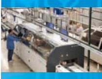
SigmaTron's investment in Surface Mount Technology netted well over 50—and growing—SMT lines. Shown is the equipment's automated wave-soldering stage for an industrial EMS program. This and other technology capabilities exemplify the higher-level automation and efficiency being driven by SII.
