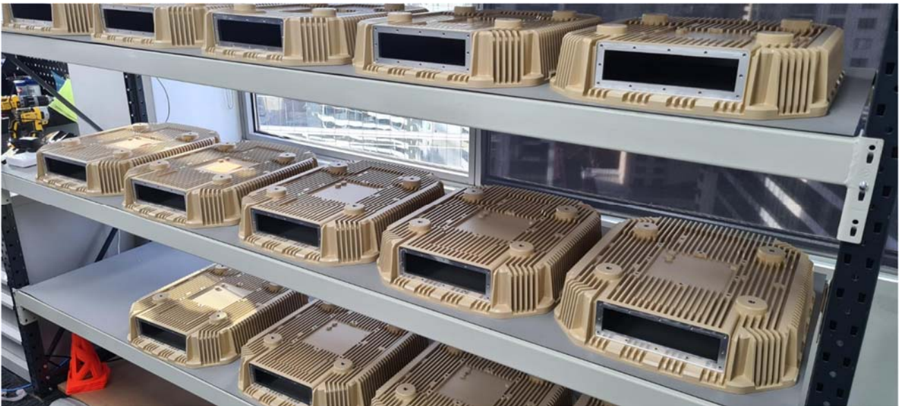
Image: DroneSentry-X™ heatsinks during the manufacturing process
