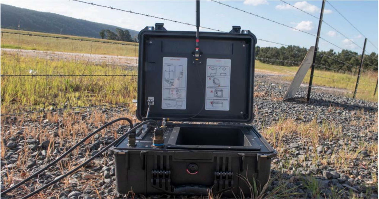
Image: DroneSim™, a lightweight and rapidly deployable UAS/drone simulator that is able to mimic common drone signals
