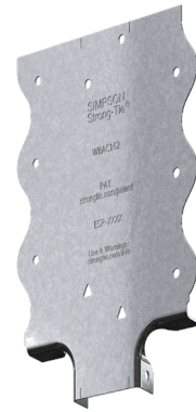
WBAC wood backing connector for attaching cabinetry and other heavy fixtures to cold-formed steel studs
