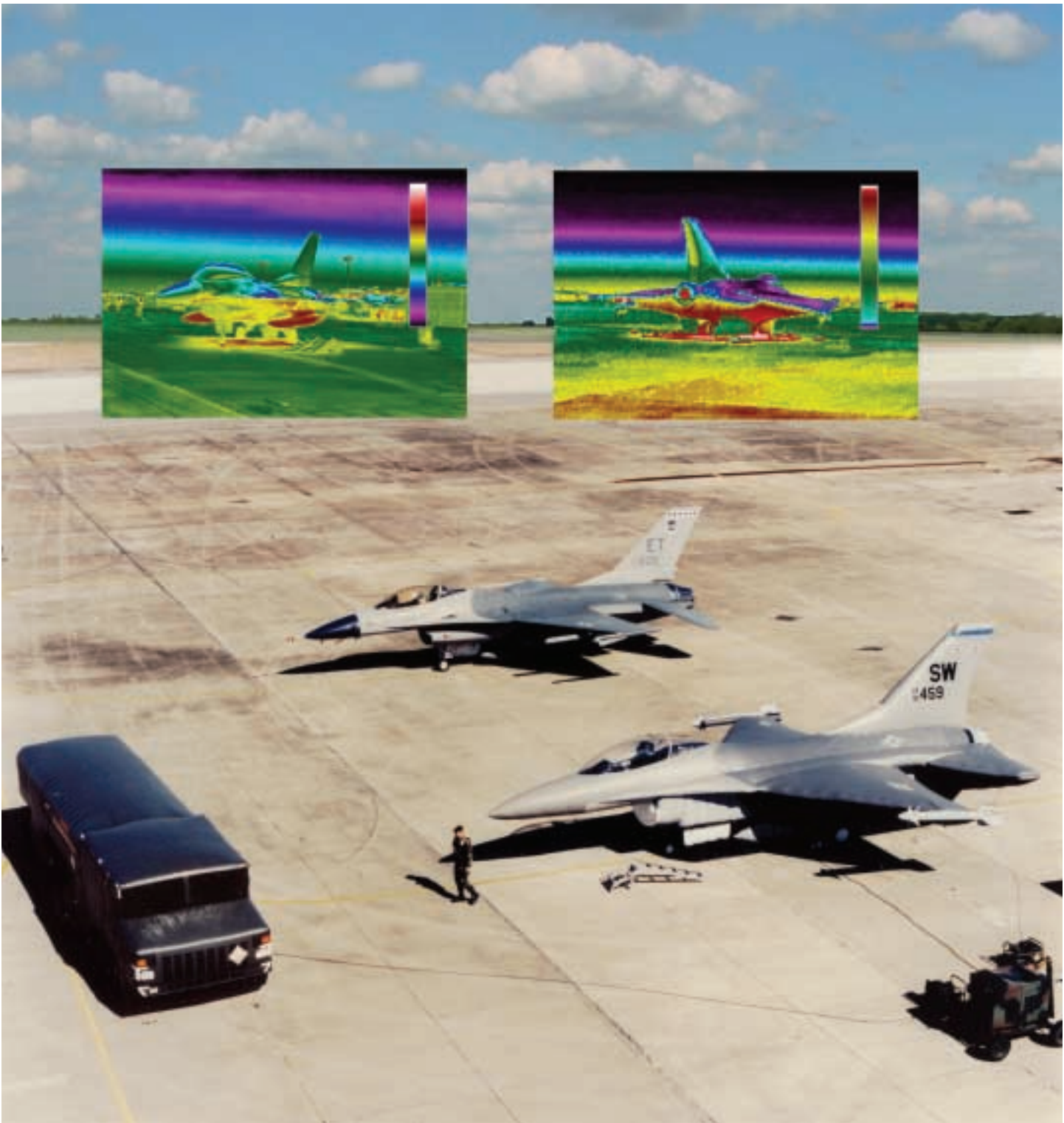
Which airplane is an inflatable? Aerostar's highly realistic inflatable decoys also mimic thermal images and radar signatures of actual military equipment.
