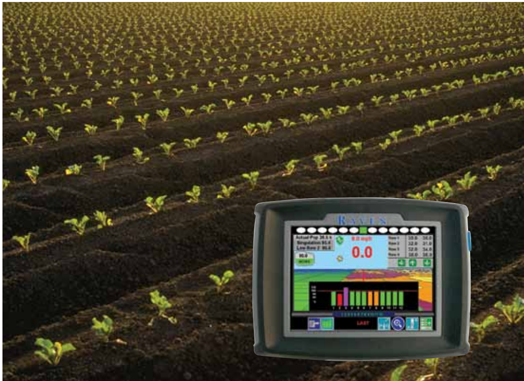
▲ The latest innovation, Slingshot™ (on left), uses wireless connectivity over cell phone networks to give cost-effective secure access to critical operating information. Raven's OmniRow™ advanced planter control system (on right) allows for variable-rate seeding and automatic section control.
