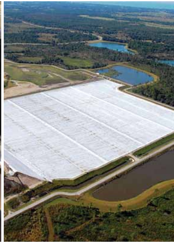
▲ Raven continues to expand with the recent addition of cast extrusion ( on left ). Our 300,000 square foot South Dakota operation produces one of the widest ranges of size, material and thickness in the industry. Raven geomembrane sheeting ( on right ) is used as a rainshed cover to divert rainwater from entering active landfills.
