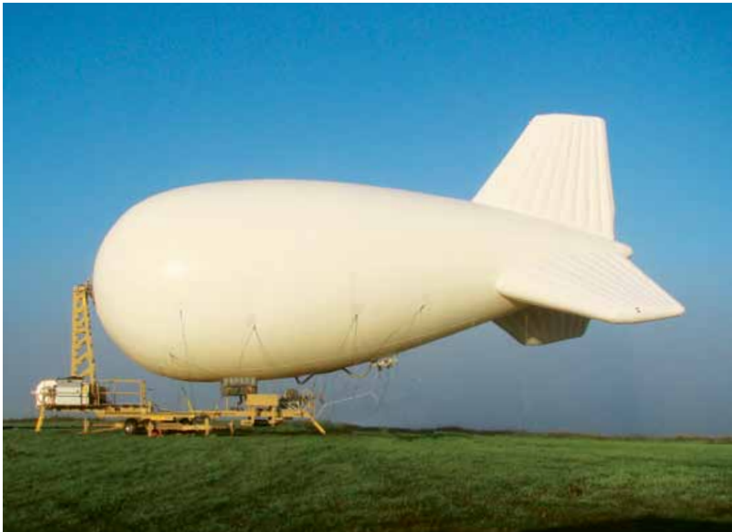
▲ Changes in the world security environment have led to a new focus on wide-area surveillance and strategic monitoring. Raven's aerostats can be flown over land or over the sea. Examples of payloads include audio and imagery surveillance, communication relay, reconnaissance and atmospheric sampling.
